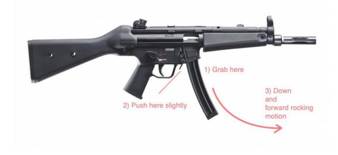
To insert magazine execute operations in the opposite direction, pushing button or paddle mag may be not necessary.
