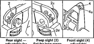
adjustable for windage and elevation Peep sight (2) Set for long range 300-800m with small aperture up Front sight (4) adjustable for zeroing only
